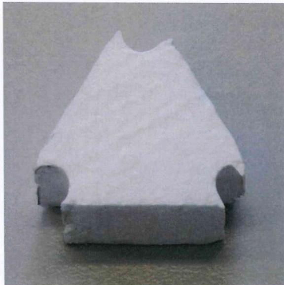
Figure 14: Triangular foam spacers for the boom
