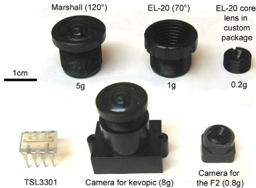
Figure 3.8: Vision chip (bottom-left), optics (top) and camera packaging (bottom center and right). Marshall and EL-20 optics are interchangeable in the camera for kevopic. In an effort of miniaturisation, the TSL3301 has been machined such to fit the small custom-developed package labelled “Camera for the F2”, whose overall size is only 10x10x8mm. The 8 pins of the TSL3301 have been removed and the chip has been directly soldered on the underlying printed circuit board. The EL-20 core plastic lens has been extracted from its original packaging and placed into a smaller one (top-right). The weight gain is fivefold (a camera for kevopic with an EL-20 weighs 4g).
